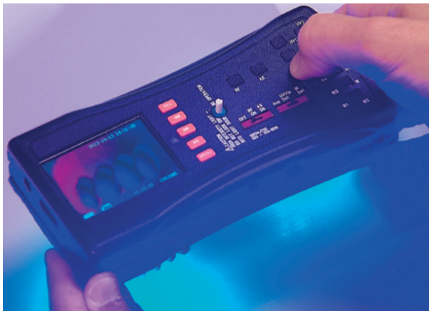
■ Authentic and counterfeit drugs being screened by CD-3, a small portable device invented by FDA scientists © U.S. Food and Drug Administration.
